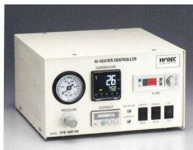
3) Temperature, air pressure, flow rate controller with over-temperature monitoring <HYK-20AF-DK>
